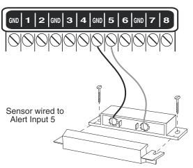
Figure 2-6. Sensor Connected to an Alert Input
