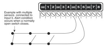
Figure 2-9. Multiple Normally Open Sensors
