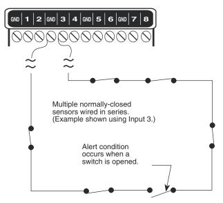
Figure 2-8. Multiple Normally Closed Sensors
