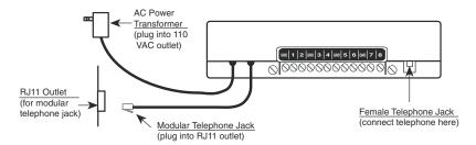
Figure 2-4. Installing the Telephone Line
