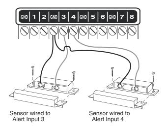
Figure 2-7. Two Sensors Wired to Adjacent Inputs
