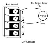
The different sensor types connected to the terminal block.
