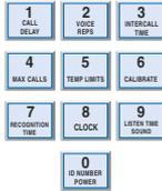
5. Position the pound (#) or asterisk (\*) within the telephone number where required by pressing SET (where the pound is located) or WHAT IS (where the asterisk is located). The Model 1108 will *beep* each time pound or asterisk is pressed.
