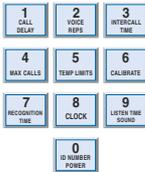
5. Press CODE. This instructs the Model 1108 to wait for the telephone call to be answered by the beeper or pager service. (A voice message will not occur—only digital tones are used.) Note that CODE may not work with beepers where there is no ring before the beeper connects. If that proves to be the case for your particular beeper, skip the CODE step and proceed from Step 4 to Step 6.
