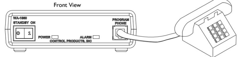
2. Push the ROCKER SWITCH on the front panel to STANDBY—alarm LED will be flashing.
