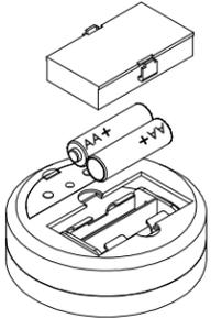
**Note:** Once the batteries are installed, leave the sensor turned upside down to mute the audible 90 dB beep, which starts in approximately 30 seconds, and beeps every 10 seconds thereafter until joined to the WA-1000 base station.
