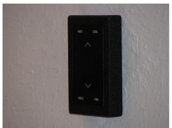
Complete installation of the Thermostat Keypad by sliding it over the anchor screws.
