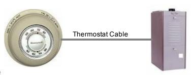
Your BAYweb Thermostat installation is shown below. The Control Module is mounted near the furnace or air conditioner and is wired into the existing thermostat cable. The control module is powered from a standard outlet.
