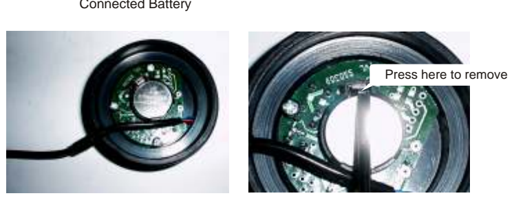
While placing Battery, see the '+' side of the battery face upwards
