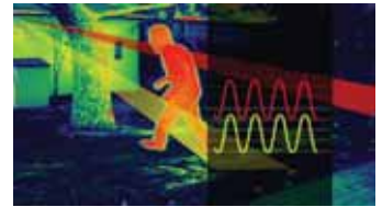
Correlated signal in both channels = PIR Alarm
