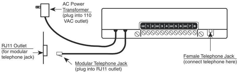
**Figure 2-4. Installing the Telephone Line**
