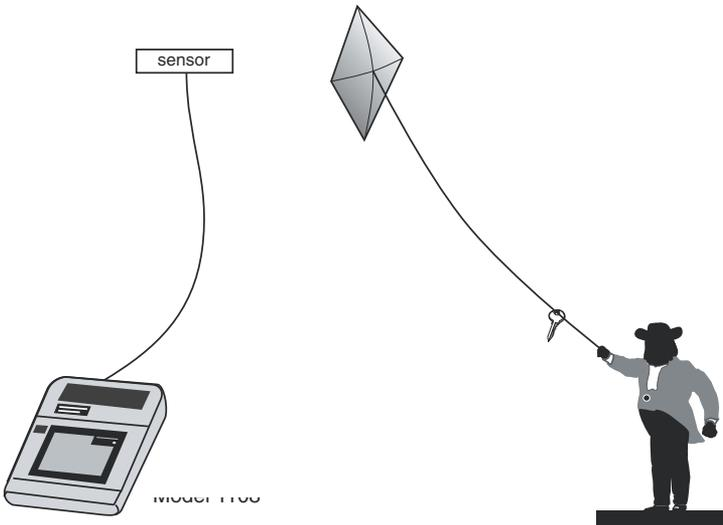
Figure 2-10. Potential Sensor Damage from Stray Electrical Noise
