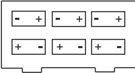
Figure 2-2. Battery Installation
