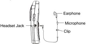
**Note:** When the headset is plugged into the headset jack the microphone on the handset will be deactivated.
