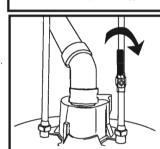
4. Position the FloodStop Valve so that the arrow on the side of the valve is pointing to the water heater. Install the FloodStop Valve between the rigid water line coming from the manual cold water valve and the
