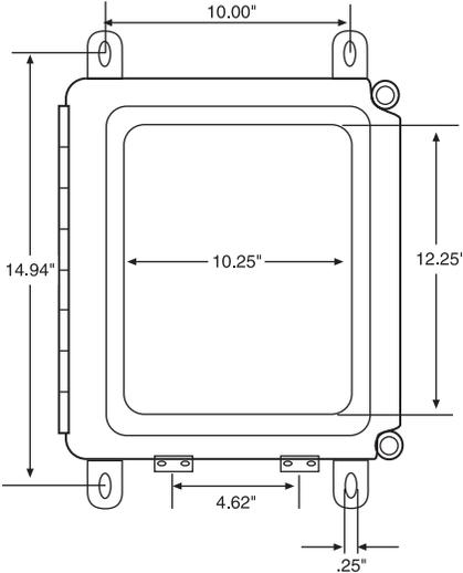
Figure 1: Mounting dimensions
